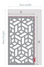
Whenever possible, the raw material sizes should be considered when planning the panel layout so that panel waste can be minimised. We support you with this.
